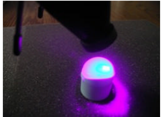
InData Scanner and Ultraviolet fluorescing optic scanning a bottle cap marked with UV fluorescing ink
