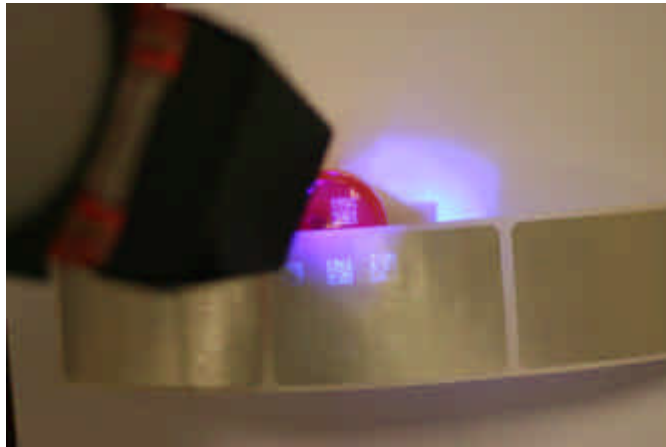
InData Systems patented UV optic illuminating “invisible” data matrix bar codes on a label. A bottle cap with UV bar code is directly behind the labels
