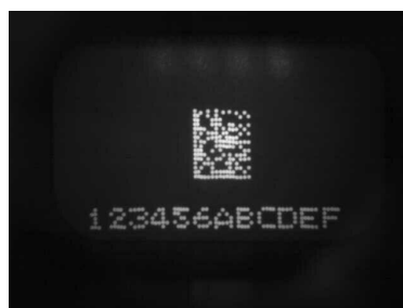
Continuous Ink Jet (CIJ) direct on products
