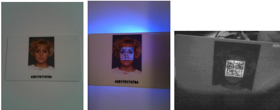
A select example of successful print behind a readable UV fluorescing bar code
